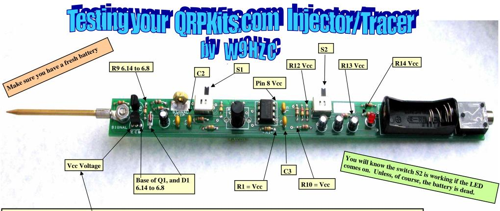
Note: With the battery installed, **measure the Emitter of Q1 first** then all the other spots labeled as Vcc. The actual Vcc voltage will be different on each Tracer because of component tolerances but it should read the same at all test points seen here.
