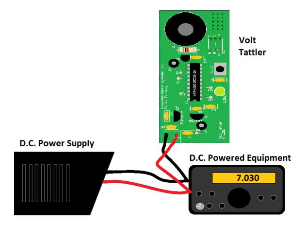
Setting up VoltTattler at the equipment can alert an operator to voltage drops between the power source and your equipment. In addition hearing the "roger" beep (Morse 'R', .-.) can audibly alert you if the power dropped out and then came back again (intermittent connection). This can be very useful in troubleshooting a system.
