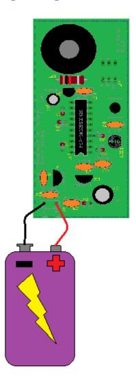
First connect the new Volt Tattler to one of the 9-volt batteries. As always watch polarity. If the battery is relatively alive the Volt Tattler should sound the Morse 'R' (.-.) then repeated Morse 'L' (.-..). In addition the heartbeat LED should flash periodically.
