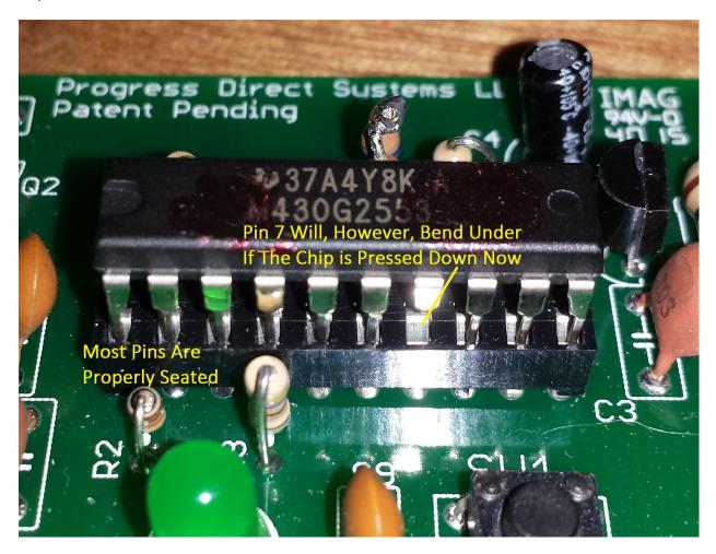
Here the builder is headed for trouble. Pin 7 of the chip is not pointing down into the socket but tucked a bot back under the chip. When they push down on the chip to seat it into the socket, pin-7 will fold under the chip and not connect. This may cause issues even though the chip seemed to seat solidly. Check each pin for proper direction before attempting to seat the chip into the socket.
