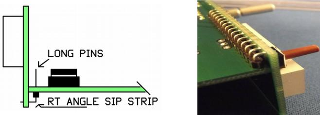
1. Insert long leads of SIP pin strip up through bottom side of main board. Make sure it is seated against the board along it's length.
