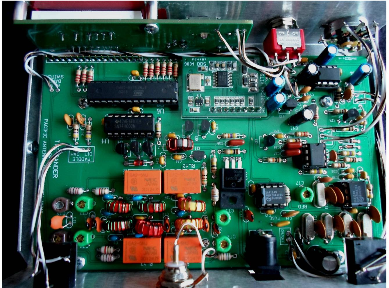
Note how wires "float" above the board.
