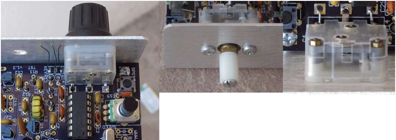
Figure 43 Mounting of C1. Mount C1 on the front panel first, then solder the leads from the top side.
