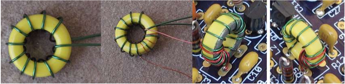
Figure 31. L2 transformer. 11T (15m) green primary, 4T red secondary
