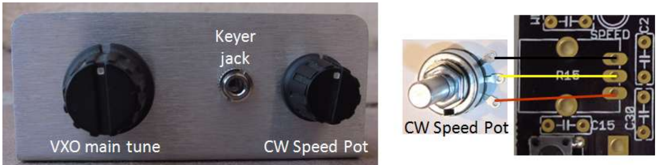
Figure 40. Panel mounted CW speed pot and visualization of PCB connections
