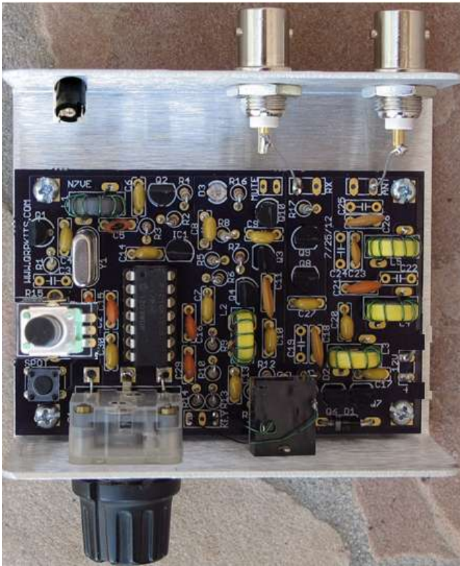
Figure 38. Completed kit in case (less connections to rear 12v power jack)
