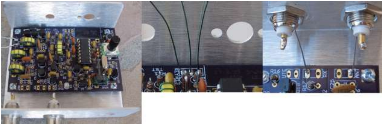
Figure 39. Mount PCB in the frame using four 4-40 screws. Add keyer leads, antenna leads
