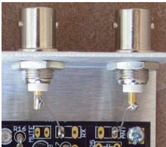
Figure 41. Transmitter antenna connection (ANT) and external receiver (RX) connection
