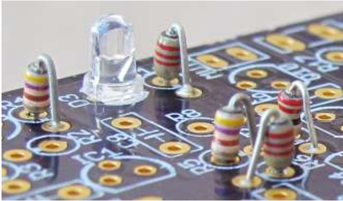
Figure 16. Resistors are mounted vertically, with short leads, body on the circle, close to the PCB
