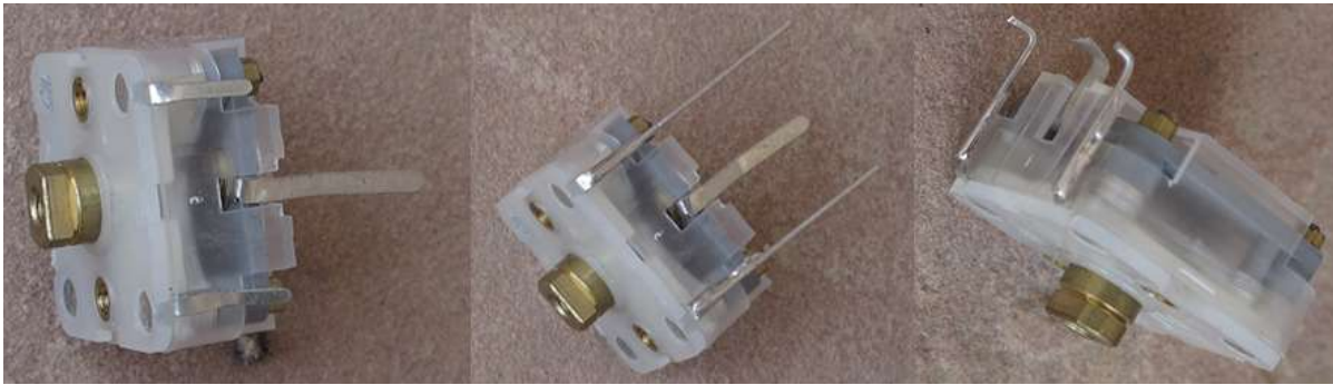
Figure 42. Polyvaricon with short leads. Leads extended with resistor leads. Form and clip leads.
