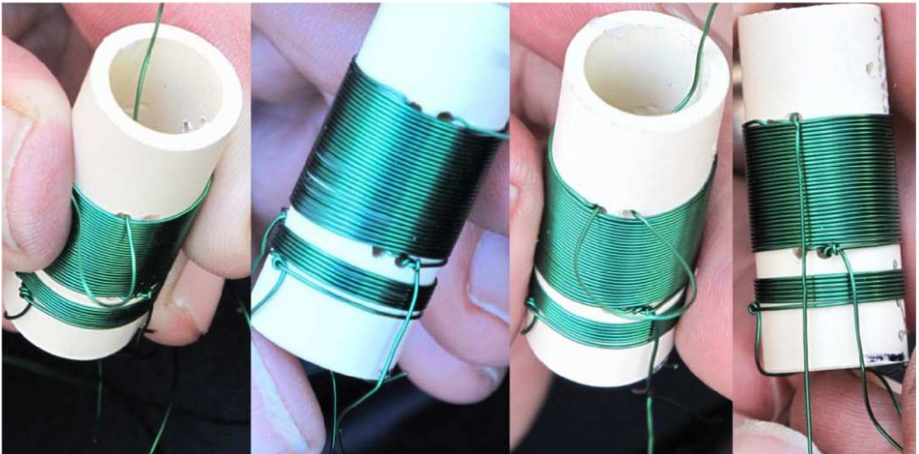
Figure 54. Tying off L1 middle winding
