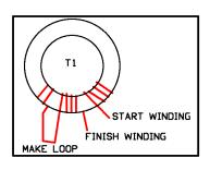
L1 and T1 are mounted on the bottom side of the board!
