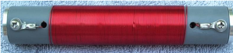
The Completed 80 meter coil
