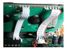
The LCD is connected to the main board via a length of ribbon cable.
