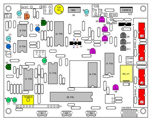
Start with the sockets. Make sure you have all the pins through the holes in the board before soldering!!! Also make sure the notch on the socket is orientated with the notch on the location outline.
