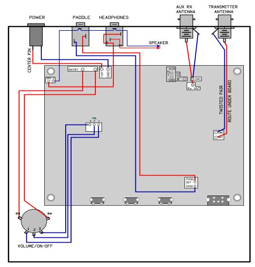
Wires connecting to volume control, the paddle jack and transmitter antenna jack should be routed under the board to keep the wires out of the way. It just looks neater this way.
