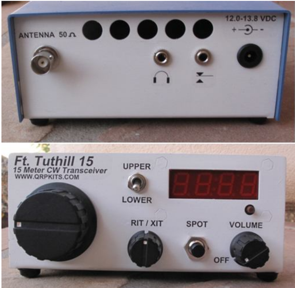
Figure 32. Picture of decal locations on the front and back panels (painted case)
