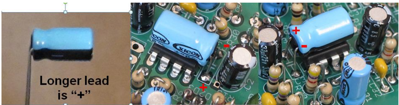
Figure 14. Lead forming and mounting for C3, the 220 uF cap.
