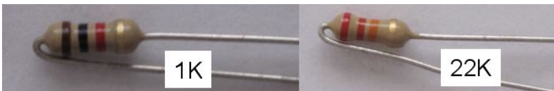
Figure 29. Identification of 1K and 22K resistors
