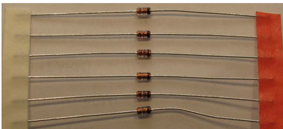
Figure 11. Picture of 1N4148 small signal diodes
