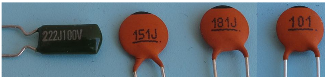
Figure 19. Identification of 100, 150, 180 and 2200 pF capacitors
