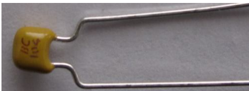
Figure 15. Picture of 0.1 uf Cap marked "104"
