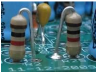
Figure 30. Resistors are mounted vertically, body on the circle, close to the PCB
