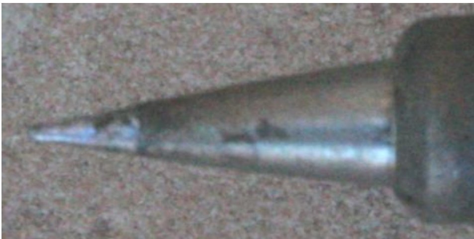
Figure 3. A very pointed soldering iron tip is a big help for small components
