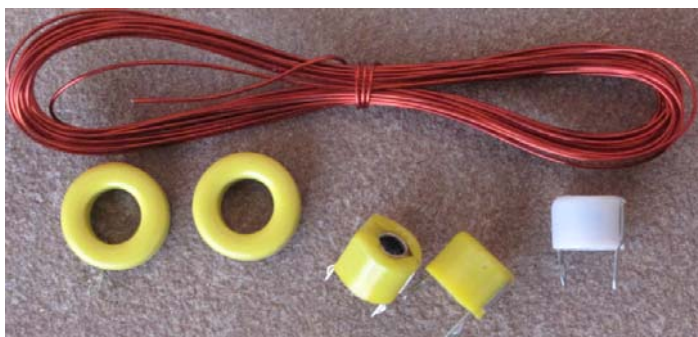
Figure 15. Mixer filter parts needed. Three trim caps, two T37-6 cores, and red enamel wire
