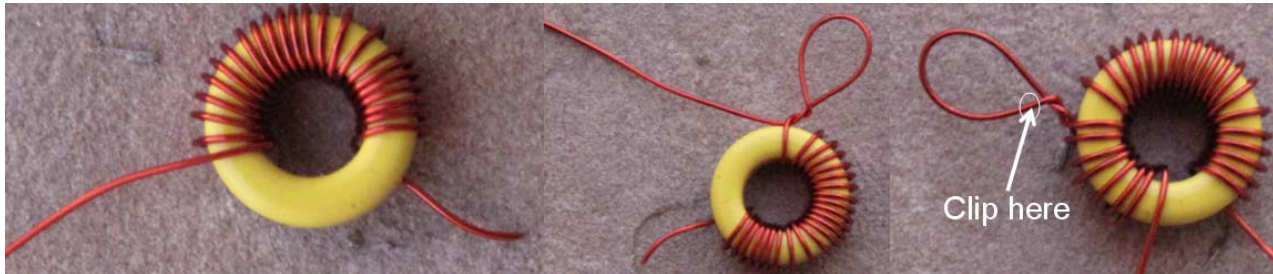
Figure 33. L9 VFO coil. 21 turns, add a tap, then wind 7 more turns to finish
