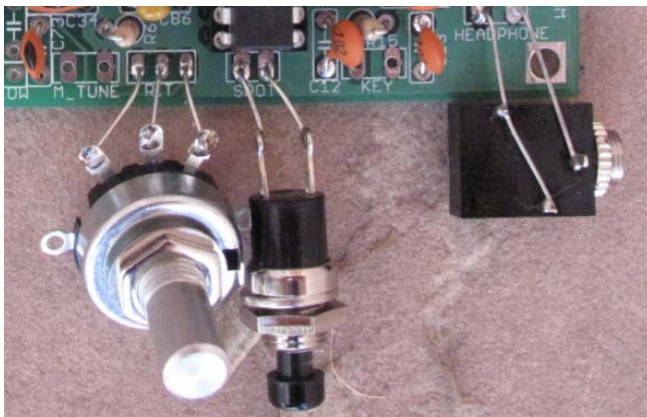
Figure 6. Temporary installation of the 10K RIT pot, SPOT switch, and Headphone jack
