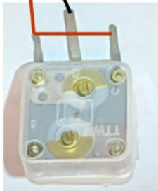
Figure 53. Connection of main tune capacitor and Hi/Low band Switch
