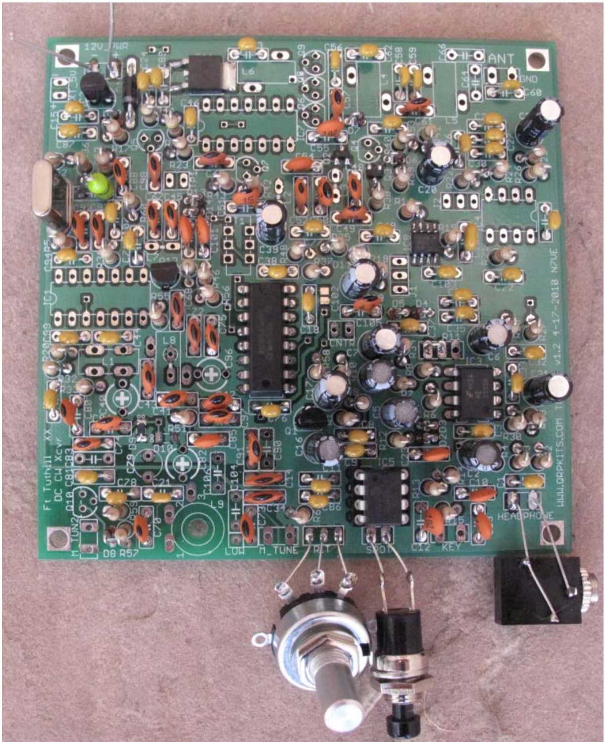
Figure 8. Board with installation of IC3, IC5, IC6, Y1 and misc test controls
