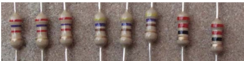
Figure 31. Identification of 2.7K, 470 and 22 ohm resistors in order left to right
