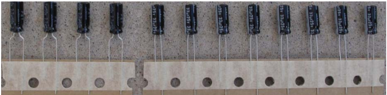
Figure 21. Identification of 2.2 uF and 33 uF caps.
