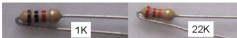
Figure 25. Identification of 1K and 22K resistors. Leads should be bent as shown for installation
