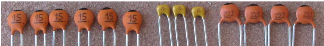
Figure 17. Identification of 15 pF, 150 pF and 22 pF caps.
