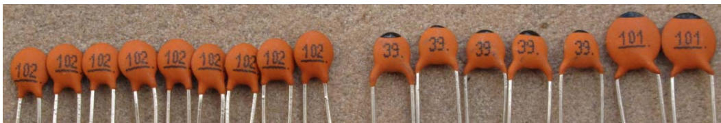
Figure 14. Identification of 39 pF, 100 pF and 1000 pF capacitors
