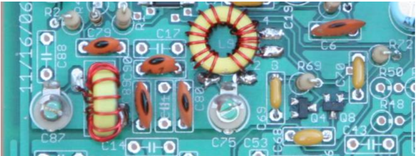
Figure 30. Close up of receiver front end and T/R switch
