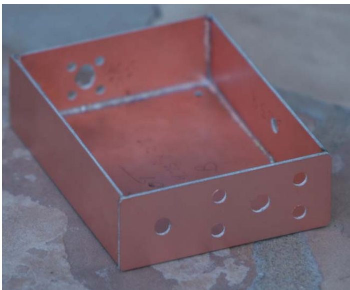
Figure 58. Homebrew case fashioned out of double sided PC board, 5" x 3.5" x 1.375".
