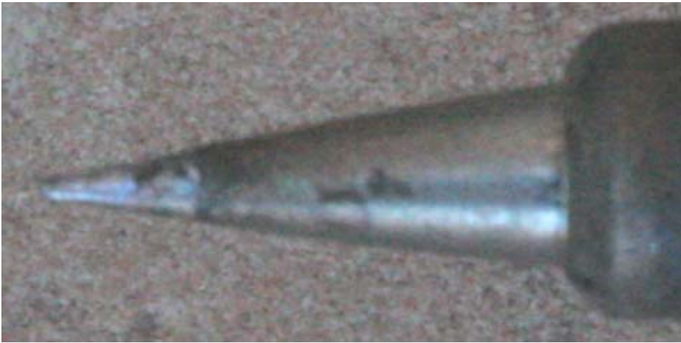
Figure 3. A very pointed soldering iron tip is a very big help for small components
