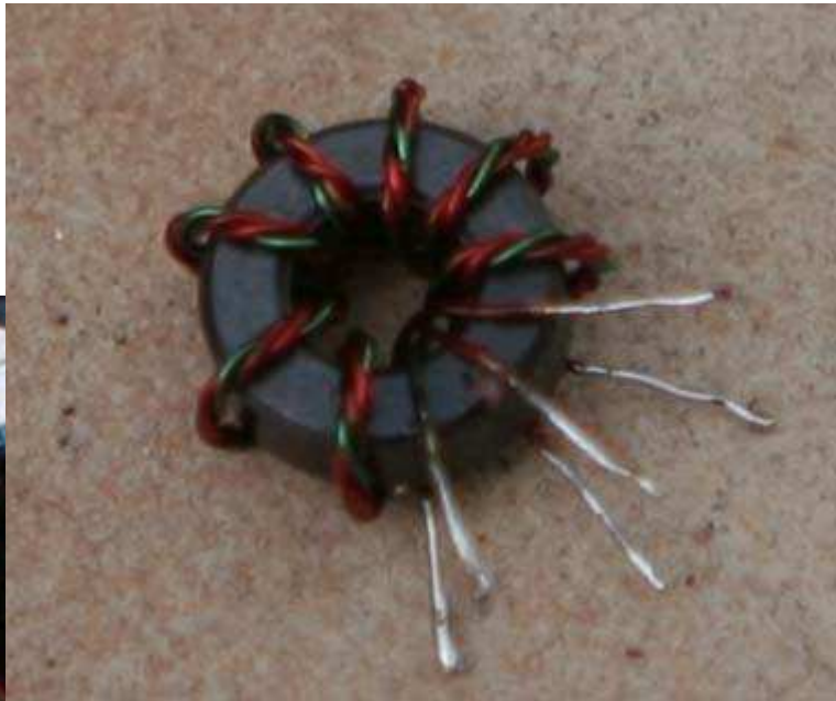
Illustration 20: T-2 Winding Detail (N7VE Photo)
