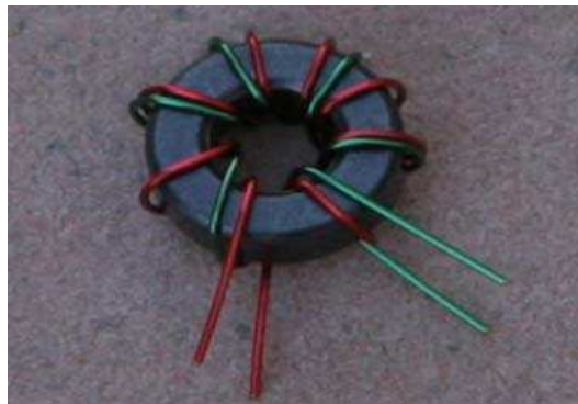
Illustration: T1 Winding Layout
