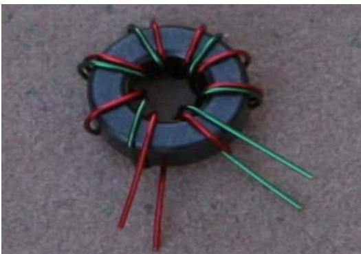
Illustration: T1 Winding Layout (N7VE Photo)
