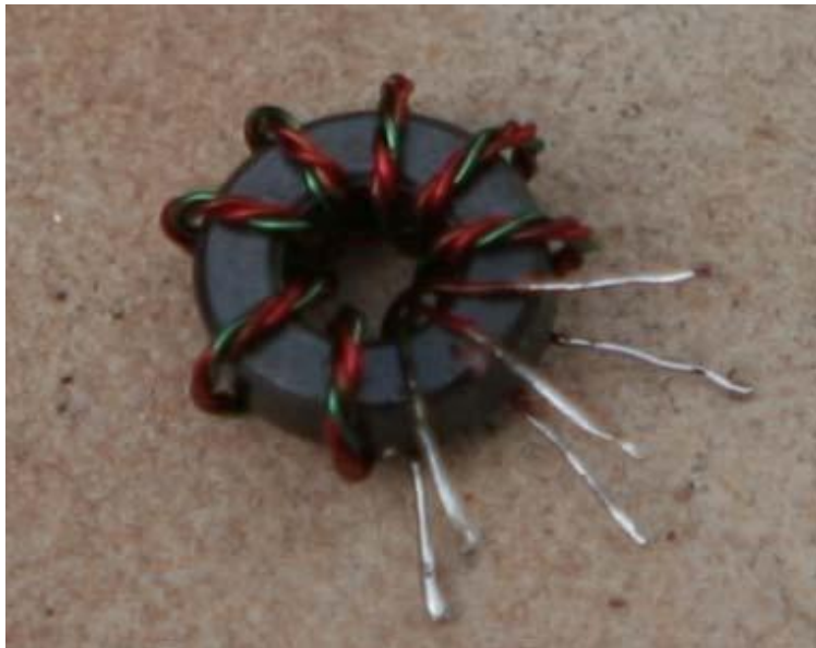
Illustration 25: T-2 Winding Detail (N7VE Photo)
