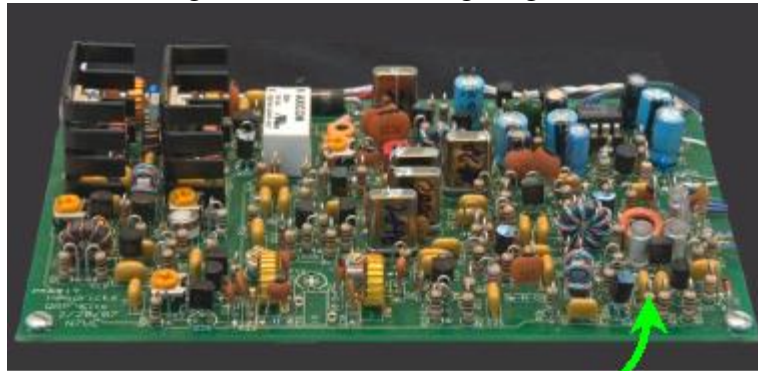
Measure VFO Frequency Here (top of R-27)
