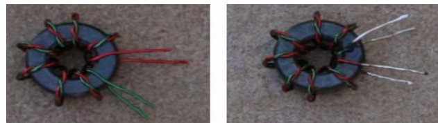
Illustration 23: T-3 Winding Detail (N7VE Photo)
