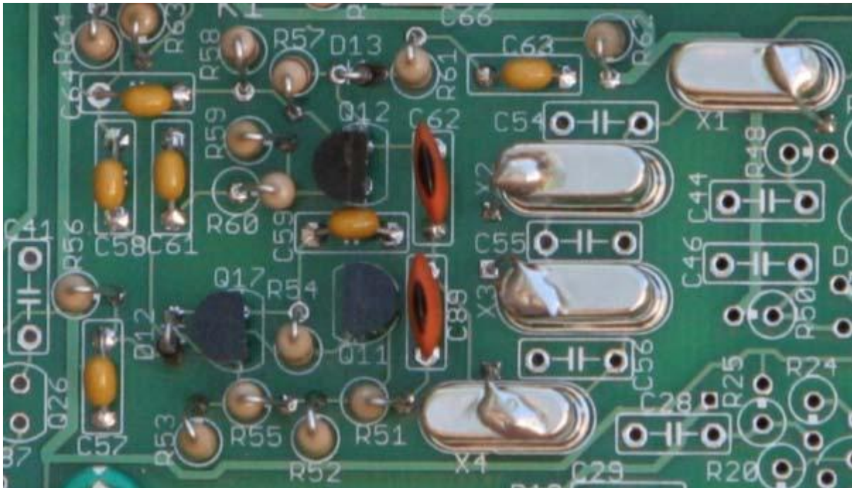
Illustration 10: Second IF Amp Section (N7VE Photo)
