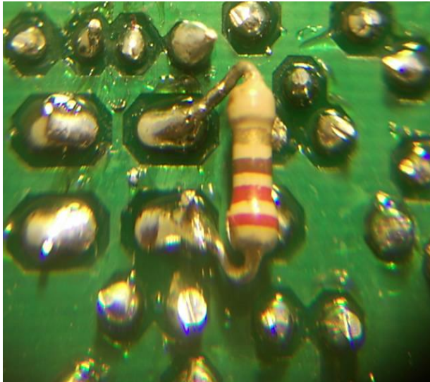
Illustration 27: 220 resistor across T-3 primary (K7HKL Photo)
