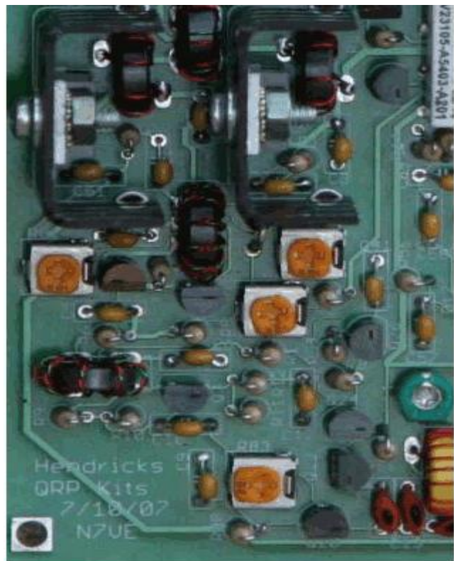
Illustration 22: RF PA Drivers (N7VE Photo)
