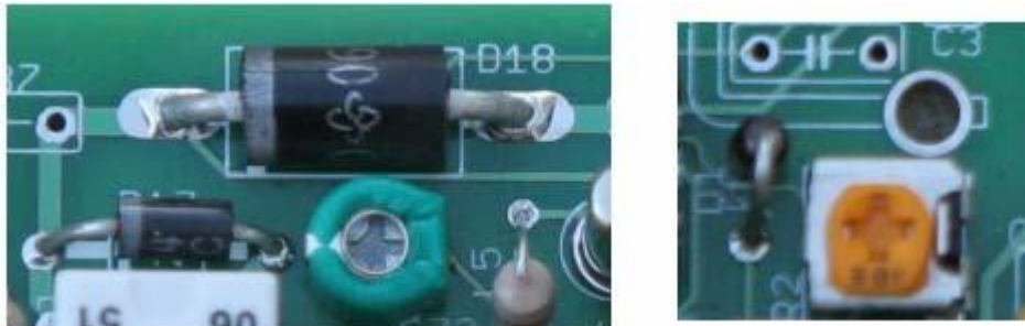
Illustration 3: D-17 and D-18 Installation (N7VE Photo)
