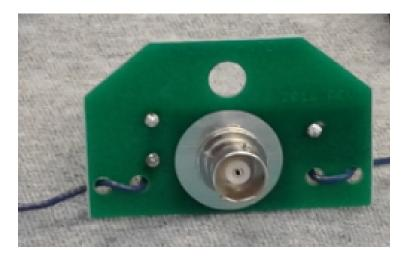
After the wire is soldered, the excess pull the excess back through the holes to secure the wire in place and prevent movement of the solder connections.
