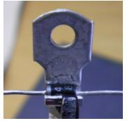
Carefully bend the leads of the diode so that they will reach down to the board when the diode is attached to the heatsink. Be careful to keep the leads from shorting to the ring terminal.
