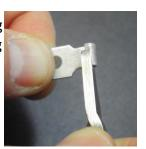
The ring terminal should fit into the u shaped area formed by opening up the crimp area on the ring terminal. Before crimping down, apply a small amount of heat sink compound to the diode body.
